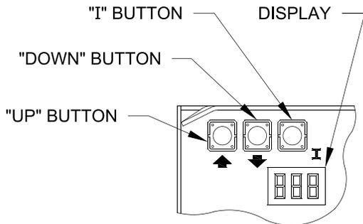
**Figure 34: Boiler Control Key Function & Orientation**
