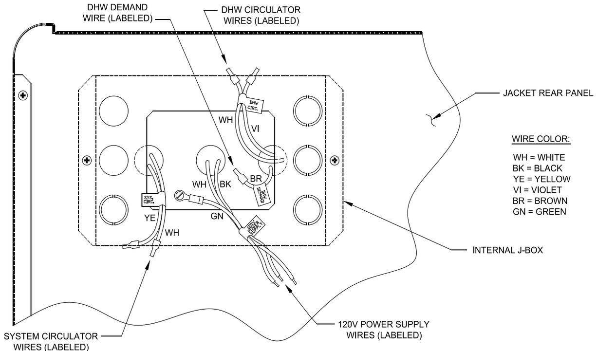
Figure 7: Internal Junction Box and Wiring Harness Details
