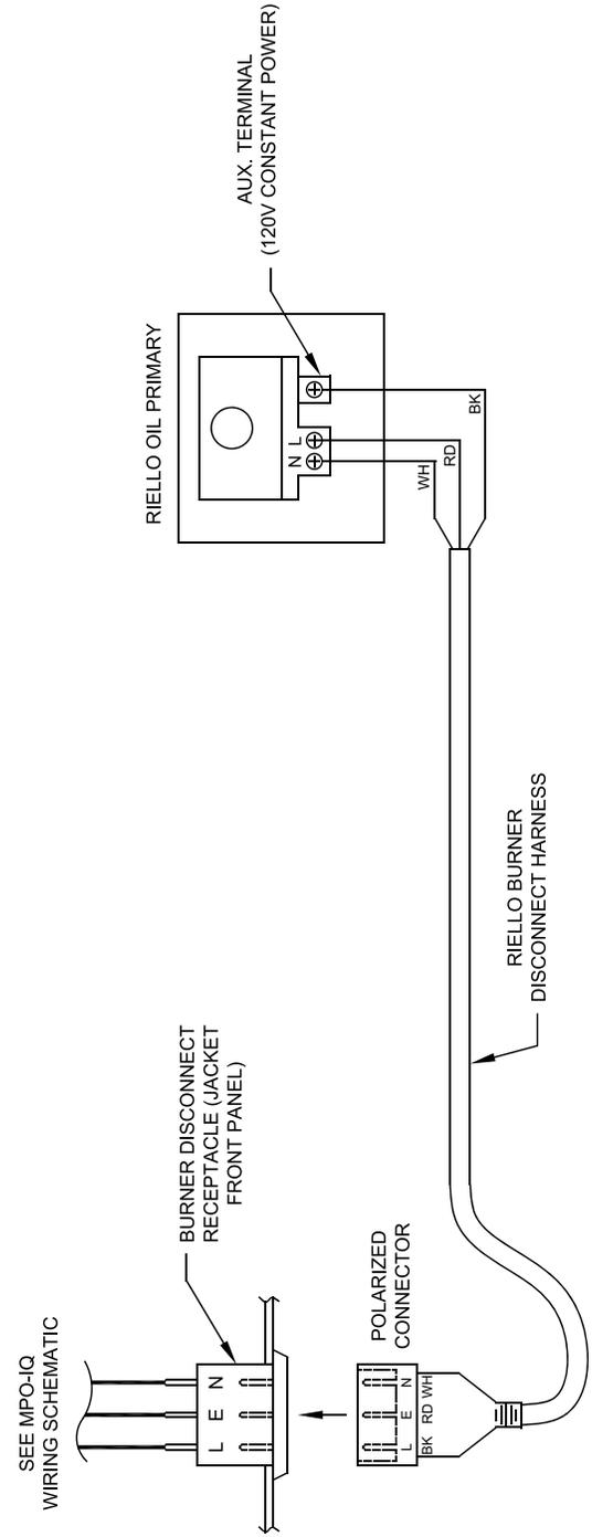
Figure 28B: Schematic Wiring Diagram, All Burner Options
