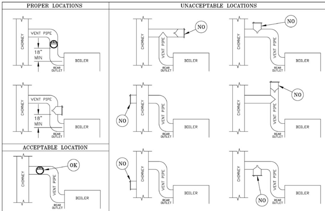
**Figure 16: Proper and Improper Locations of Draft Regulator**
