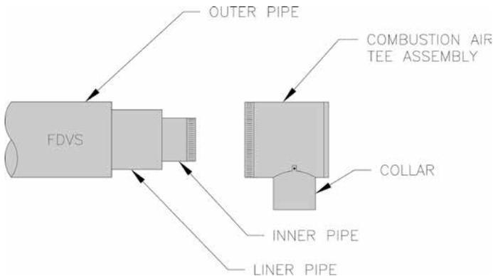
**Figure 21: Combustion Air Tee Assembly Installation**
