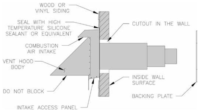
**Figure 20: Vent Hood Body Installation**
