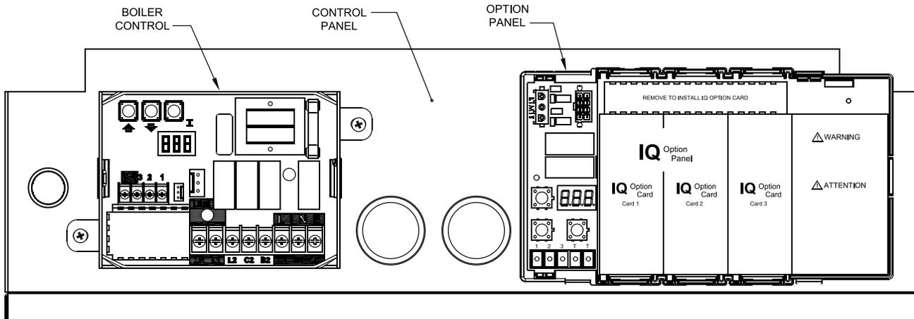
**Figure 33: Boiler Control & Option Panel Orientation**
