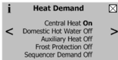
This screen provides the status of the boilers five (5) possible heat demands. When demand is off the Control has not detected the call-for-heat. This screen allows the user to determine which demands are present when more than one demand is present.
